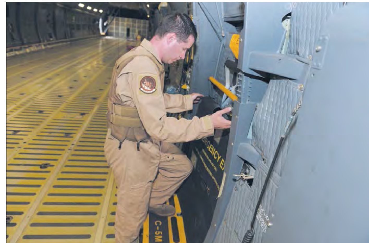
U.S. Air Force photo/Tech. Sgt. James Hodgman Tech. Sgt. David Bass, 22nd Airlift Squadron C-5M Super Galaxy loadmaster, affixes armor Sept. 12 to the inside of one of the troop doors of a C-5 at Travis Air Force Base, Calif. The armor is required to ensure air crew safety while the aircraft fly's through hostile environments.
